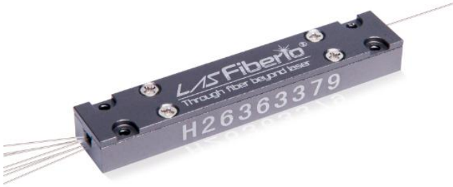
Fig.1 P23: 65x12x7.5mm 信号功率<50W
